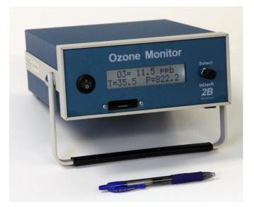
The 2B Technologies Model 202 Ozone Monitor<sup>™</sup> is designed to enable accurate and precise measurements of ozone ranging from low ppb (precision of ~1.5 ppb) up to 250,000 ppb (250 ppm) based on the well-established technique of absorption of UV light at 254 nm. The Model 202 Ozone Monitor<sup>™</sup> is lightweight (5.5 lb, 2.5 kg) and has a low power consumption (12V DC, 0.60 amp, ~7.2 watt) relative to conventional instruments and is therefore well suited for applications such as:
