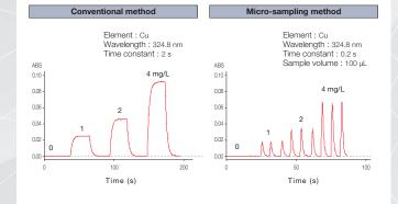
Since the baseline is stable, the method of micro sampling can be effectively carried out.
