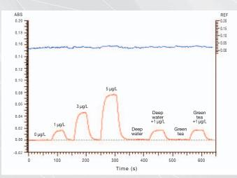
The baseline is stable immediately after turning on the hollow cathode lamp, and an arsenic concentration levels of 1  $\mu g/L$  can be readily measured.
