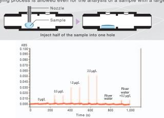
Antimony concentration levels of 0.2  $\mu g/L$  contained in river water can be measured without concentrating by heating.
