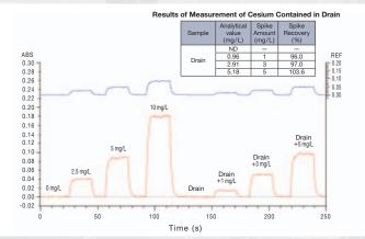
Even for cesium, which has a long absorption wavelength (852.1 nm), accurate background correction can be achieved.
