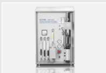
The **ONH-2000** is ideally suited for the quick simultaneous determination of oxygen, nitrogen and hydrogen in steel, cast iron, molybdenum, nickel, copper, zirconium, titan, ceramics and other inorganic samples.
