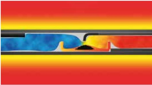
The horizontal resistance furnace of the CS-580 | CHS-580 is equipped with a ceramic combustion tube and silicon carbide heating elements. Full electronic control of the furnace ensures maximum service life of the components, including current limitation during heating-up. A sensor monitors ambient temperature and provides data for automatic reference point compensation of the thermo control, ensuring that the furnace temperature remains unaffected by fluctuations of the ambient temperature.
