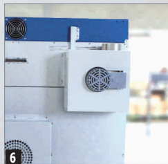
6 Air cooling extractor
